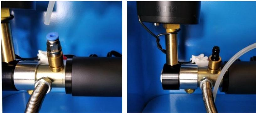
A source bottle hose is connected to this coupling, the pressure which will be multiplied goes into the booster and is filled into a target bottle or airgun connected to the outlet hose.
