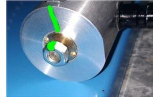
The outlet pressure from the regulator is very important and in case of exceeding the maximum allowed outlet pressure, the silicone hose will rupture, which serves as a burst-fuse and protects the booster from damage due to excessive pressure. **Never replace this hose with another hose, there is a risk of damage to the booster and injury to the operators !!**
